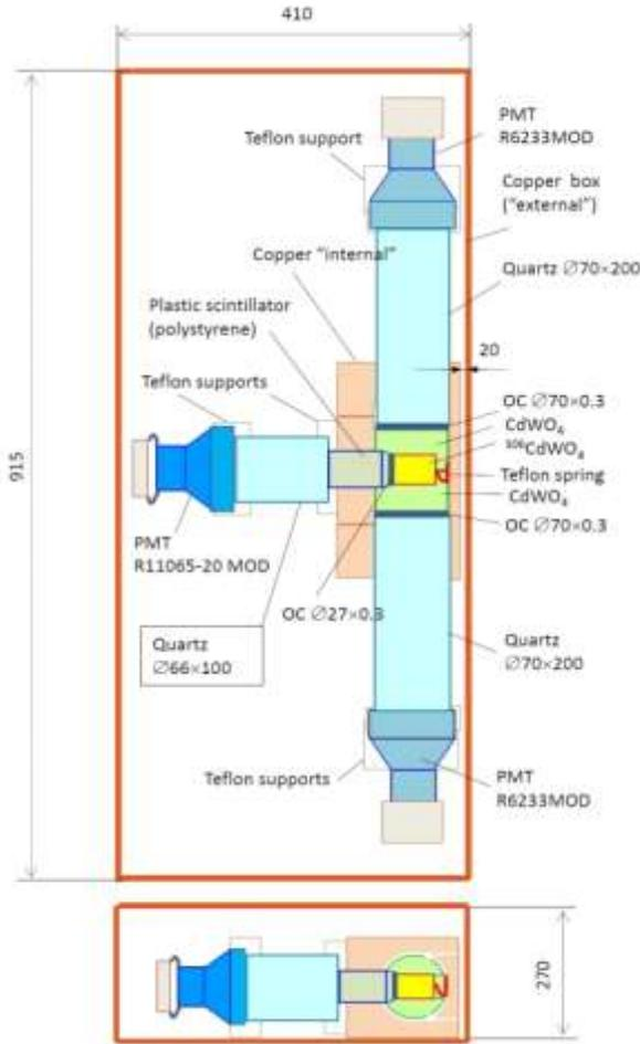
Fig. 2. Schematics of the experimental set-up. PMT is photomultiplier tube. OC is for optical couplant
