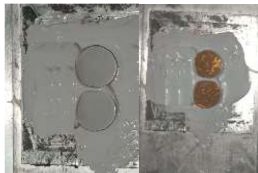
Fig. 4. The spinel samples before irradiation (left) after irradiation (right)
