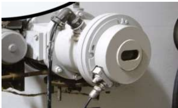
Fig. 1. Electron output unit of the M-30 microtron
