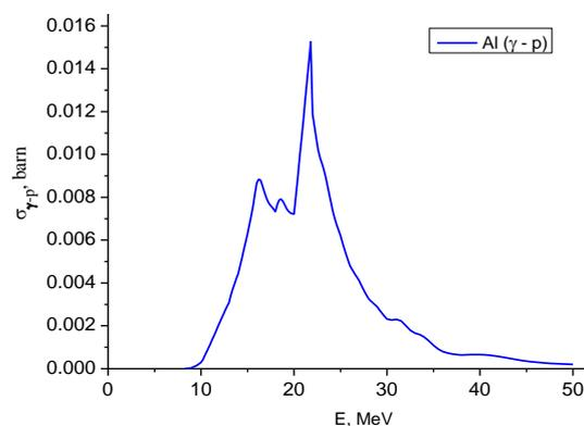
Fig. 2. The cross-section of the reaction  $^{27}\text{Al}(\gamma-p)^{26}\text{Mg}$  in aluminum
