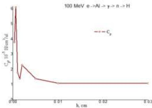
Fig. 4. Profile of hydrogen deposition in the aluminum film
