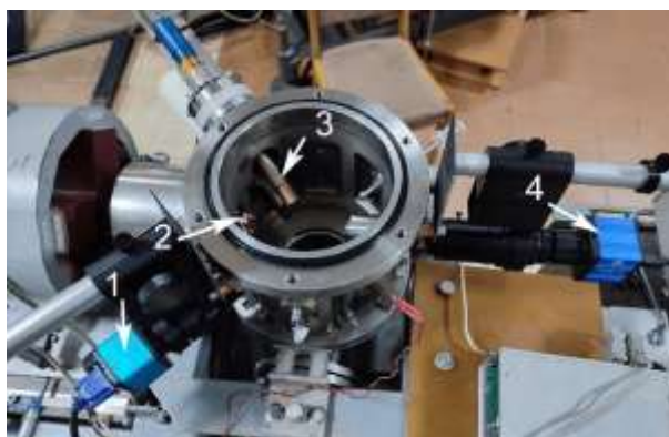
Fig. 2. Exterior view of the target chamber with the installed equipment. 1 – front video camera; 2 – LED backlight; 3 – XRD detector; 4 – rear video camera
