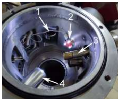
Fig. 3. Internal view of the camera with the installed equipment. 1 – location of the front video camera for positioning monitoring; 2 – LED backlight; 3 – CBR detector; 4 – location of the rear video camera for focusing
