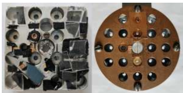
Fig. 1. Exterior of the old (left) and new (right) sample holder in the target chamber
