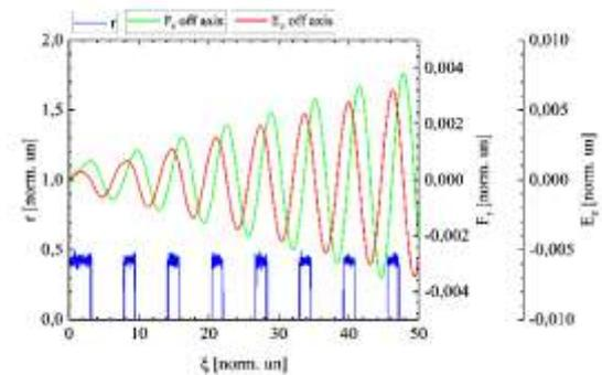
*Fig. 1.  $E_z$  (red),  $F_r$  (green) and  $r$  (blue) for the resonant sequence of eight uniform bunches with length  $l_b = \lambda/4$  (except the first one, which has length  $l_b = \lambda/2$ ). This figure shows distribution at  $z = 3$ . Here and below, we use the axial coordinate system  $(r, \xi = z - ct)$ . To demonstrate fast radial dynamics of bunches we chose the initial Lorentz factor of the electron bunches equal 5*
