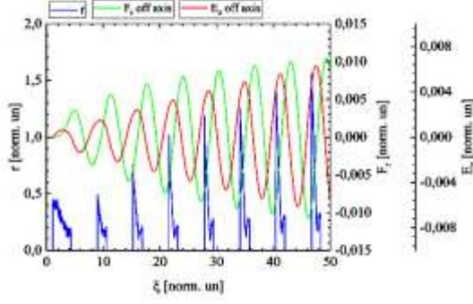
Fig. 2.  $E_z$  (red),  $F_r$  (green) and  $r$  (blue) for the resonant sequence of eight uniform bunches with length  $l_b = \lambda/4$  (except the first one, which has length  $l_b = \lambda/2$ ). This figure shows distribution at  $z = 60$
