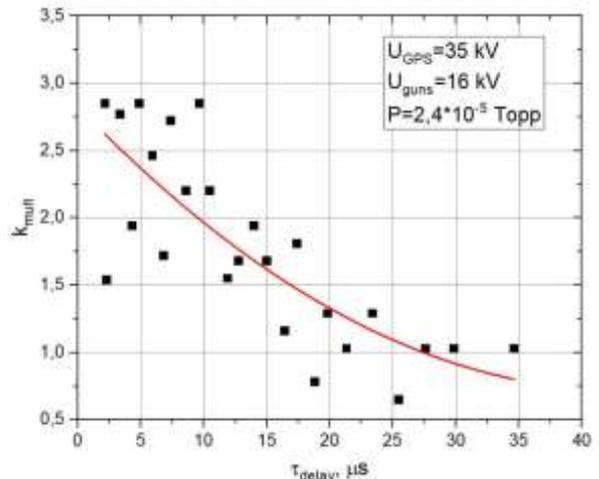
Fig. 12. The effect of delay time on the value of the multiplication factor
