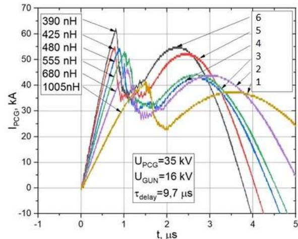
Fig. 8. The effect of inductance on the current value of the main circuit and the angle of the curve during POS operation
