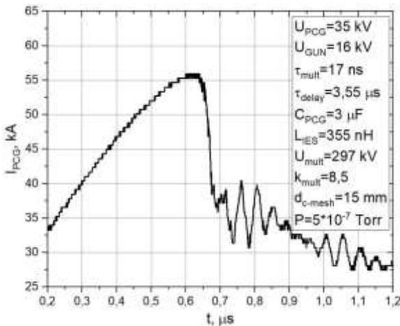
Fig. 5. Oscillograms of the main circuit current with the POS tripping
