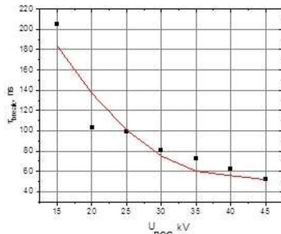
Fig. 7. Dependence of the POS opening time on the main circuit voltage
