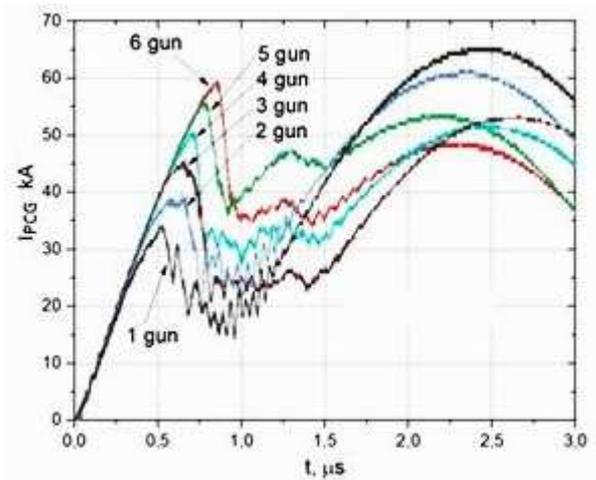
Fig. 11. Time dependence of the main circuit current for different plasma guns' number used to power the POS
