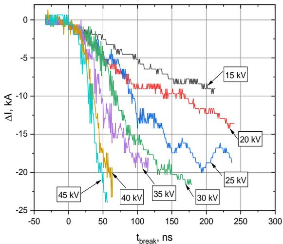
Fig. 4. Change rate of the POS current (in time of current interruption) for different PCG voltages
