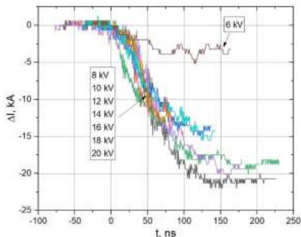
Fig. 10. Change rate of the POS current (in time of current interruption) for different plasma gun voltages
