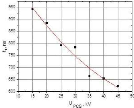
Fig. 9. Dependence of energy accumulation time on the charging voltage of the main circuit
