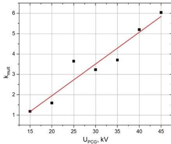
Fig. 6. Dependence of the multiplication factor on the main circuit voltage
