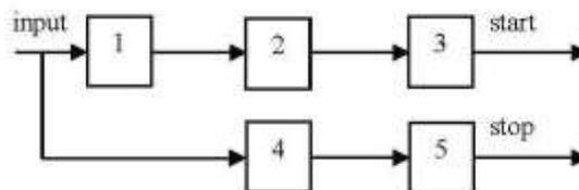
Fig. 1. The measurement setup for studying the discrimination capability (the  $FOM$ -value) of organic scintillation materials: 1 is a level discriminator, 2 is a delay circuit, 3 is a pulse shaper "start", 4 is a zero-crossing detector, and 5 is a pulse shaper "stop"
