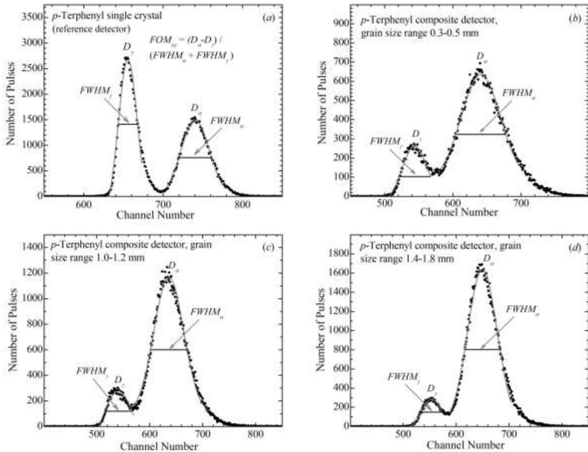
Fig. 3. Typical spectra obtained using the "zero-crossing" method for the *p*-terphenyl single crystal and *p*-terphenyl composite scintillators when excited by an alpha-particles and photons of gamma radiation from <sup>239</sup>Pu source. Other symbols are the same as in Fig. 2
