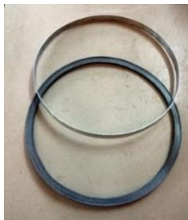
Fig. 6. Lead vacuum sealing
