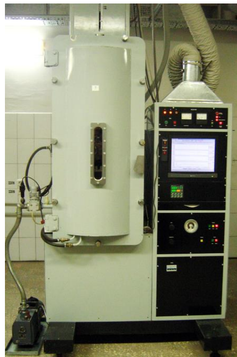
Fig. 1. Induction heating growth installation “Oxide”
