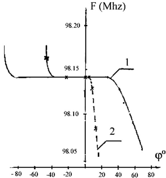
Fig. 5. Basic frequency of the resonator accelerator as a function of back coupling signal phases: 1 -  $F_{res} = f(\varphi_{FPBC})$ ; 2 -  $F_{res} = f(\varphi_{SPBC})$ .
