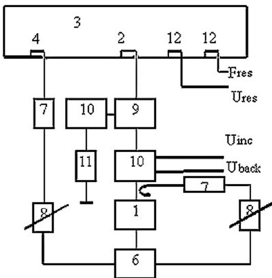
*Fig. 1. Block diagram of the self-excited generator of RF power supply of the single-section linear ion accelerator.*
