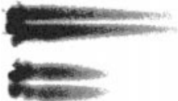
Fig. 7. Image of the Xe target made in X-rays at various currents of the central conductor.
